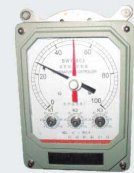
Thermometer It indicates the liquid temperature near the top of tank.
