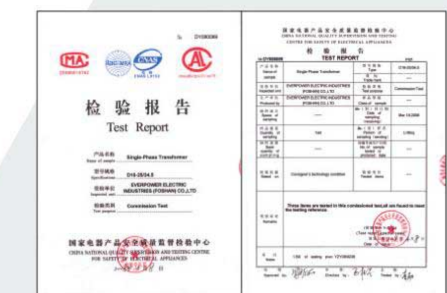
Single phase 25KVA type test from Independent Test Lab (Primary Voltage: 34.5/19.92kV)
