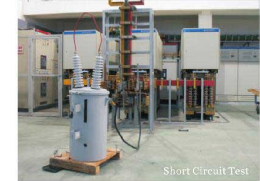
Short Circuit Test
