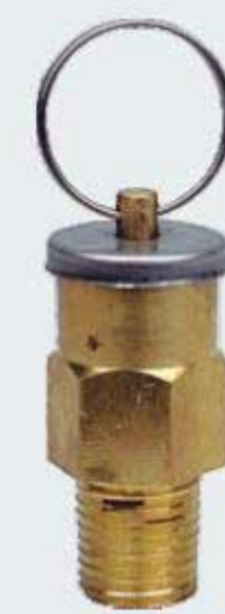
Pressure Relief Device The standard Pressure Relief Device, located on the tank above the liquid level, relieves excessive internal tank pressure and reseals at a lower positive pressure.
